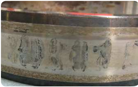
Moisture corrosion on the inner ring of a cylindrical roller bearing
