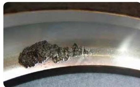
Subsurface initiated fatigue on an angular contact ball bearing outer ring raceway
