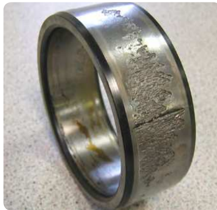
Fatigue fracture Fatigue fracture of a cylinder roller bearing inner ring
