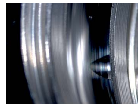
Ball indentation in raceway
