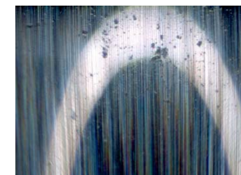
Indentations in raceway caused by particles
